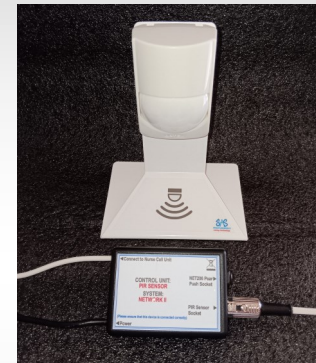
Floor Standing PIR motion detector for bed egress detection
