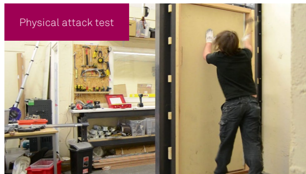
Department of Health test to simulate kicking and punching
