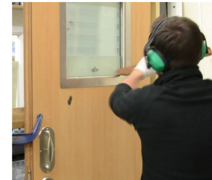
Vision panel and beading attack – to ensure robustness of the glass in the face of extreme abuse
