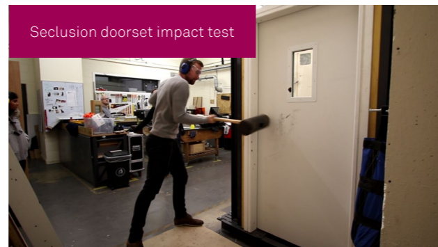
Built to withstand extreme and persistent abuse, our seclusion room door was hit more than 100 times with a paving maul in the same location
