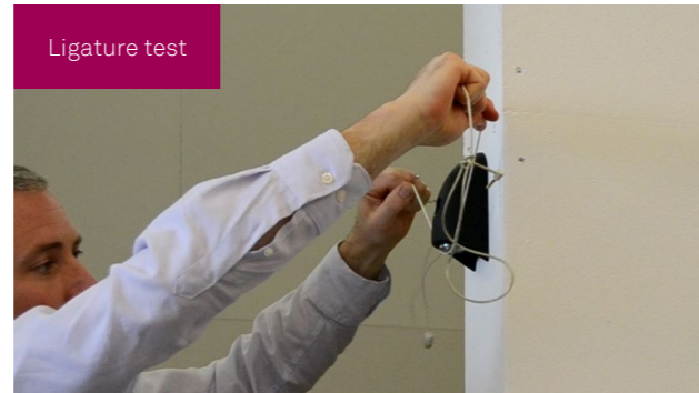
Designed to withstand extreme abuse, the en-suite pivots are tested beyond the levels set by current industry guidance
